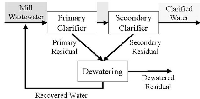
Figure 2. Pulp and paper mill wastewater treatment process.
