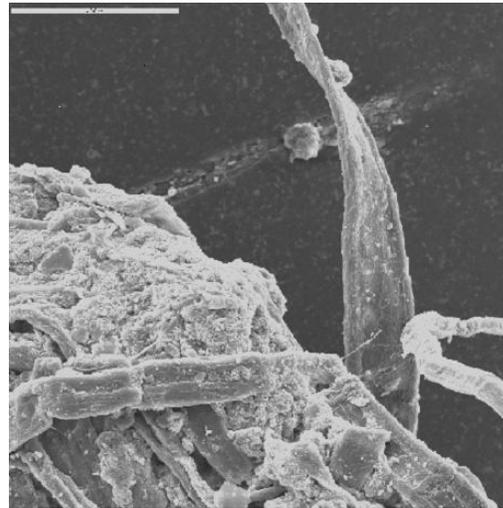
Figure 4. Pulp and paper mill sludge, 500X magnification.
