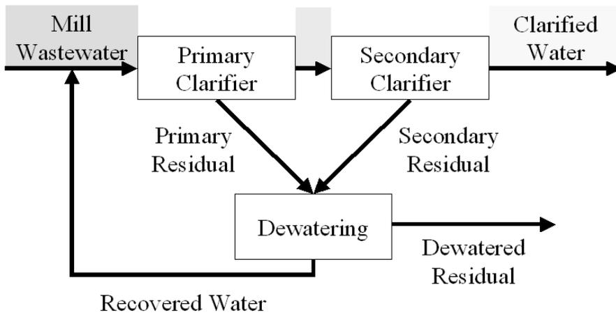
**Figure 2. Pulp and Paper Mill Wastewater Treatment Process**
