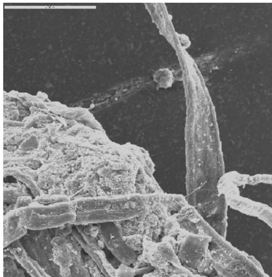
**Figure 4. Pulp & Paper Mill Sludge, 500X Magnification**
