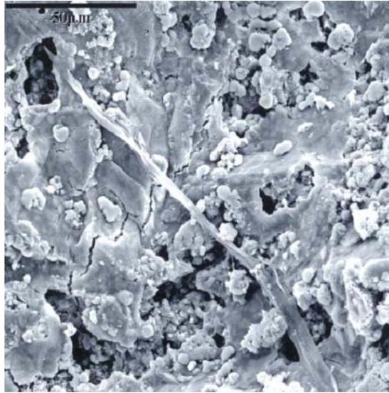
**Figure 5. Sludge Fiber Reinforcing a Micro-Crack in Concrete**
