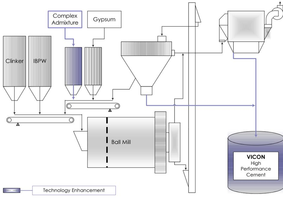
Fig. 2 - High-Performance Cement Technology
