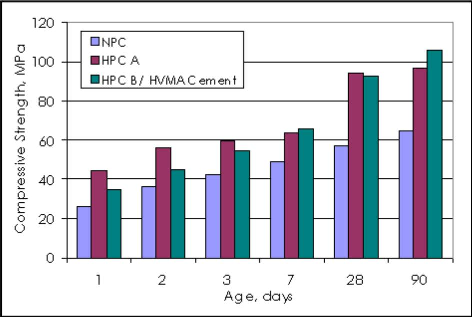
Fig. 3 - HP/HVMA Cement Strength Development
