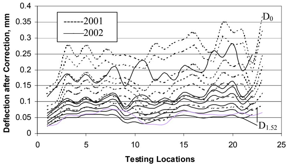
Figure 1–Pavement Deflection from FWD Test after Temperature Correction
