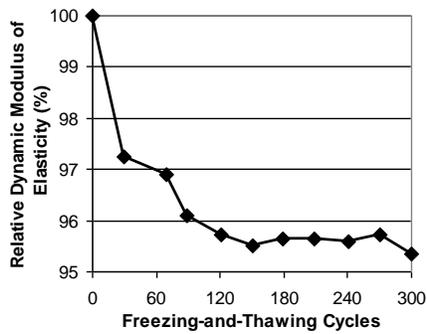
**Fig. 8 – Freezing-and-thawing resistance of concrete used for field demonstration.**
