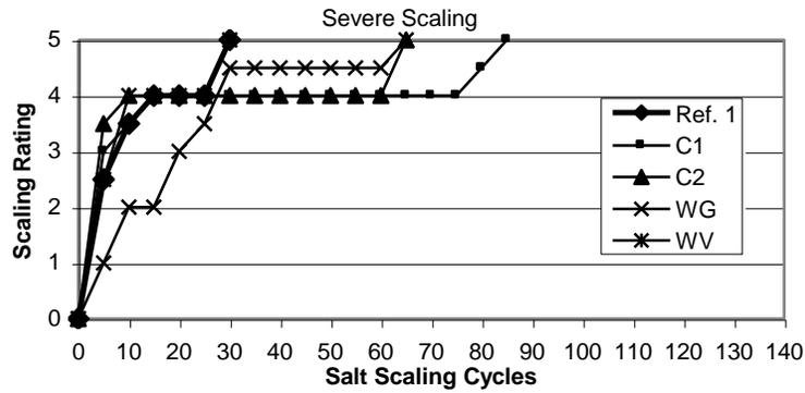
**Fig. 6 – Salt-scaling of concrete (C1, C2, WG, WV)**
