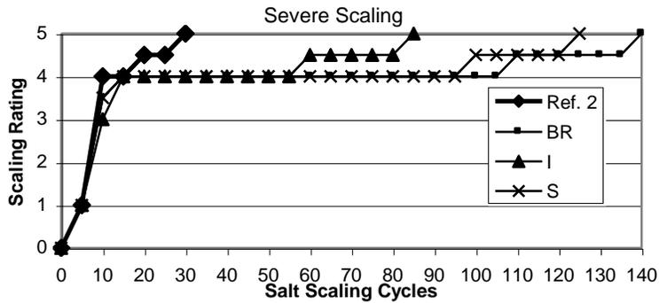
**Fig. 7 – Salt-scaling of concrete (BR, I, S)**
