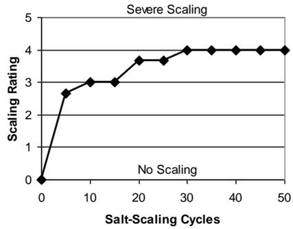
**Fig. 9 – Salt scaling of concrete used for field demonstration.**
