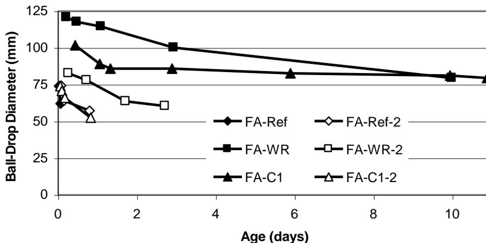
Figure 1. Ball-drop diameter on fly ash flowable slurry.
