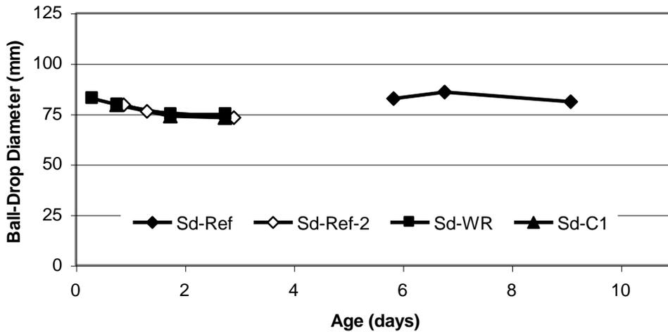
Figure 2. Ball-drop diameter on sandy flowable slurry.
