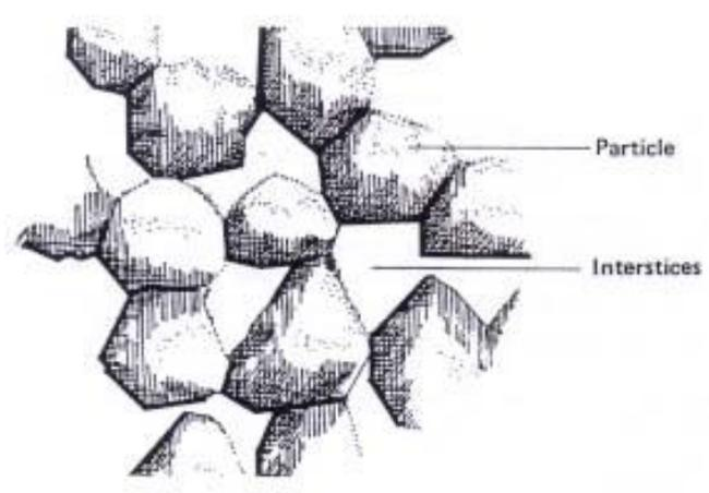
Fig. 2 - Schematic of interstices in composting material (Diaz et al., 1993)
