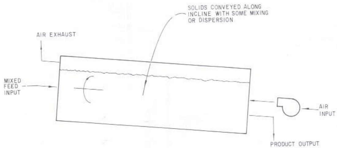
**Fig. 5 - Tumbling solids bed reactor, rotating drum or kiln (Haug, 1993)**
