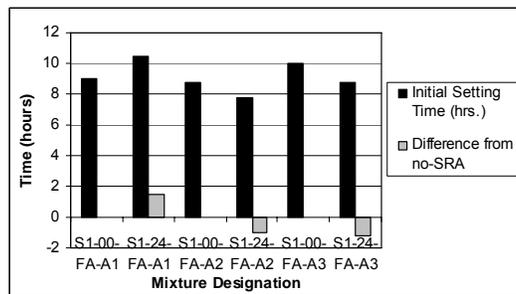
Fig. 1. Time of initial setting of concrete
