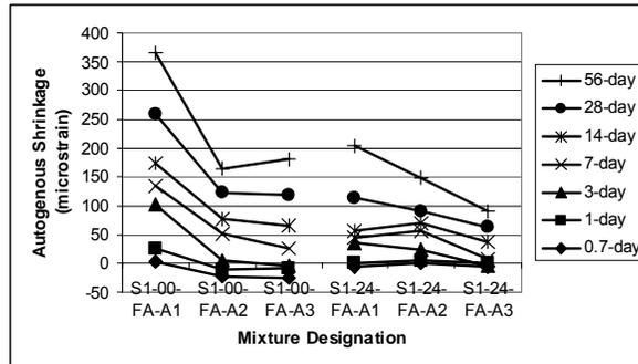
Fig. 3. Autogenous shrinkage of Grade A-FA fly ash concrete vs. aggregate type (Aggregates A1, A2, A3)
