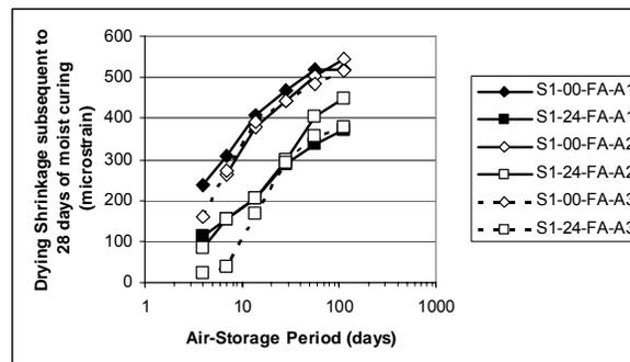
Fig. 4. Drying shrinkage of Grade A-FA fly ash concrete made with three sources of aggregates vs. age (Aggregates A1, A2, A3)
