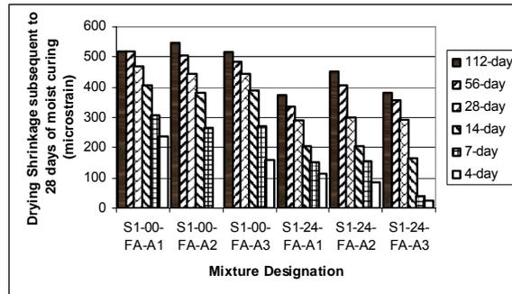
Fig. 5. Drying shrinkage of Grade A-FA fly ash concrete vs. aggregate type (Aggregates A1, A2, A3)
