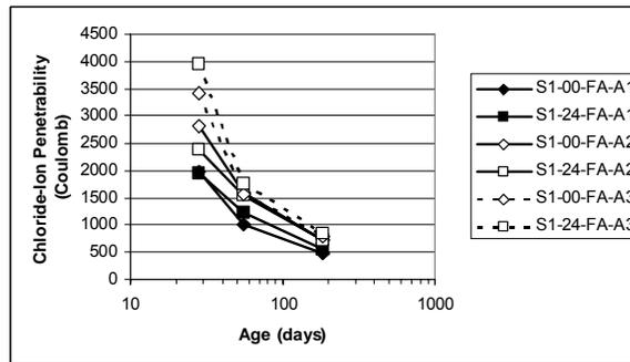
Fig. 6. Chloride-ion penetrability into Grade A-FA fly ash concrete made with three sources of aggregates vs. age (Aggregates A1, A2, A3)
