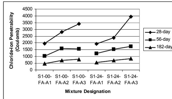
Fig. 7. Chloride-ion penetrability into Grade A-FA fly ash concrete vs. aggregate type (Aggregates A1, A2, A3)
