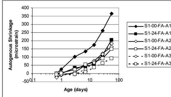
Fig. 2. Autogenous shrinkage of Grade A-FA fly ash concrete made with three sources of aggregates vs. age (Aggregates A1, A2, A3)
