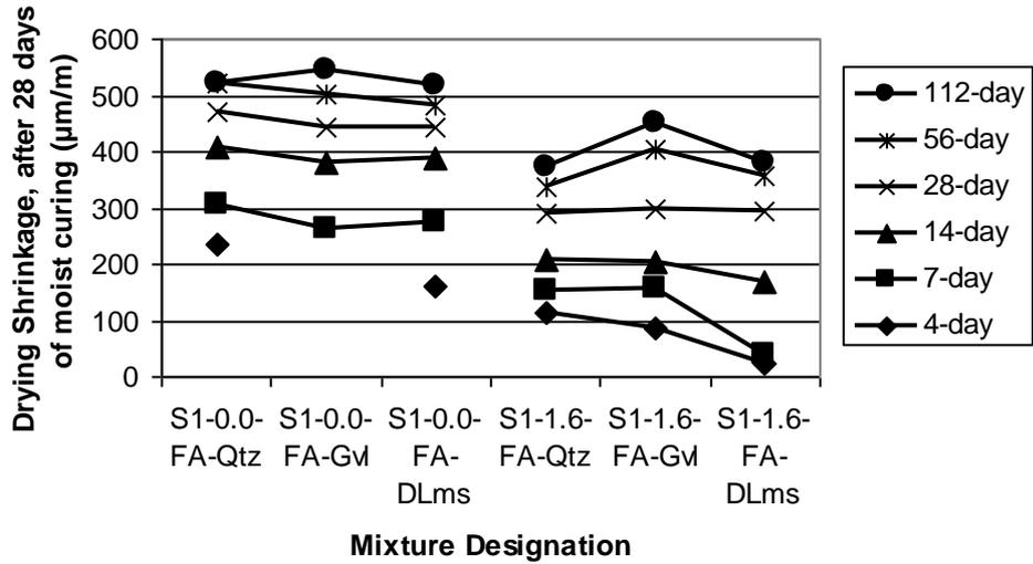
Fig. 3 – Drying shrinkage of concrete vs. aggregate type (Aggregates Qtz, Gvl, DLms).
