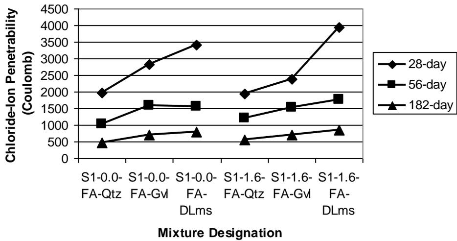
Fig. 4 – Chloride-ion penetrability into concrete vs. aggregate type (Aggregates Qtz, Gvl, DLms).
