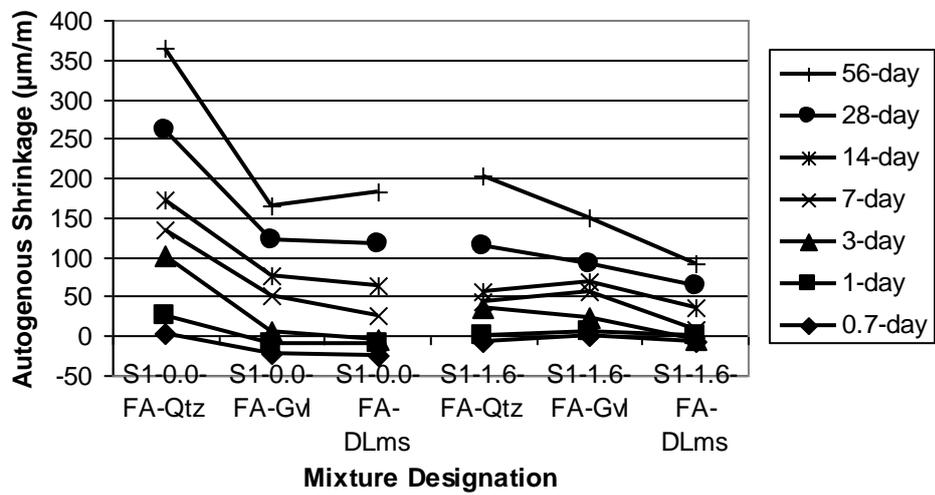
Fig. 2 – Autogenous shrinkage of concrete vs. aggregate type (Aggregates Qtz, Gvl, DLms).
