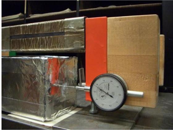
Fig. 1 – Testing of a hardened, sealed beam for autogenous length-change
