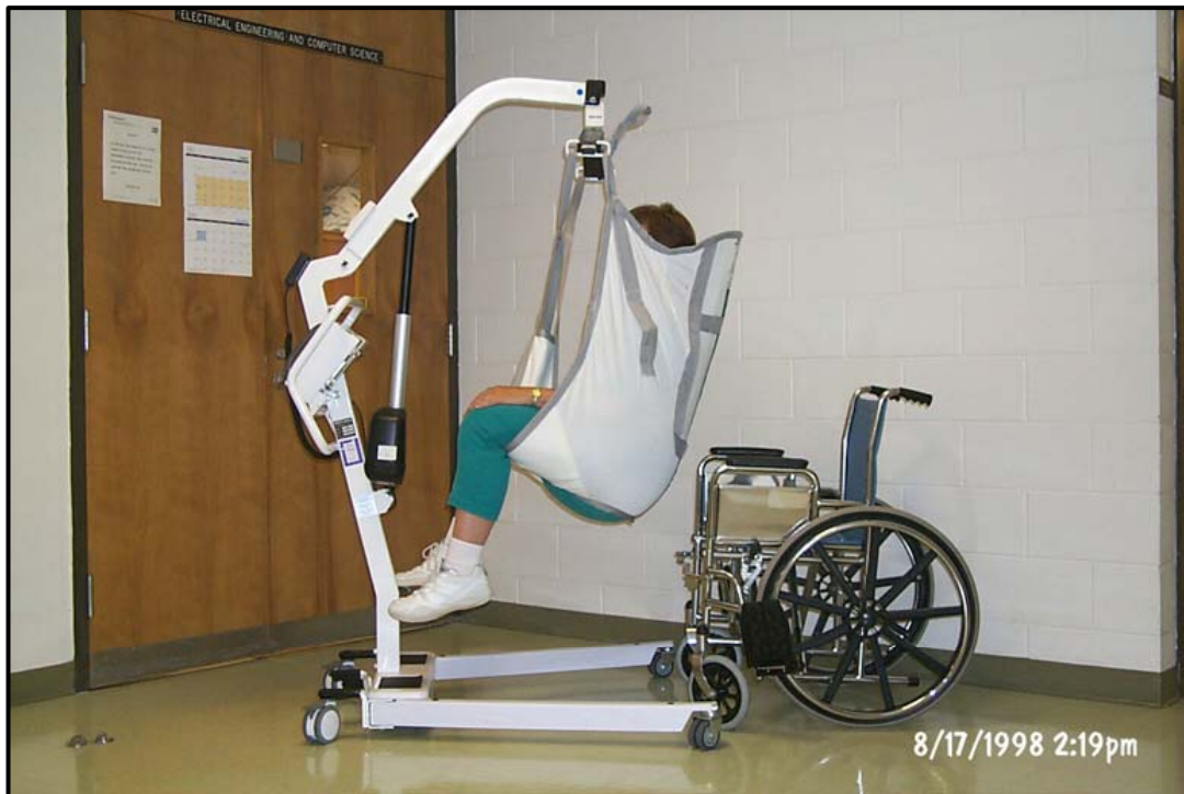
Figure 6: An example of a total lift hoist used by the nursing homes.
